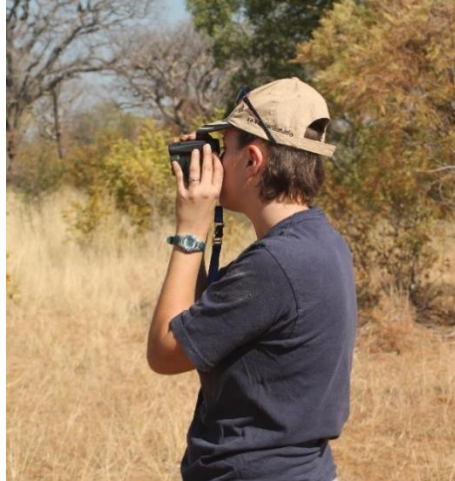
Figure 8: Field tree height measurements taken with a Vertex laser
