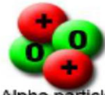
Alpha particle: 2 protons & 2 neutrons
