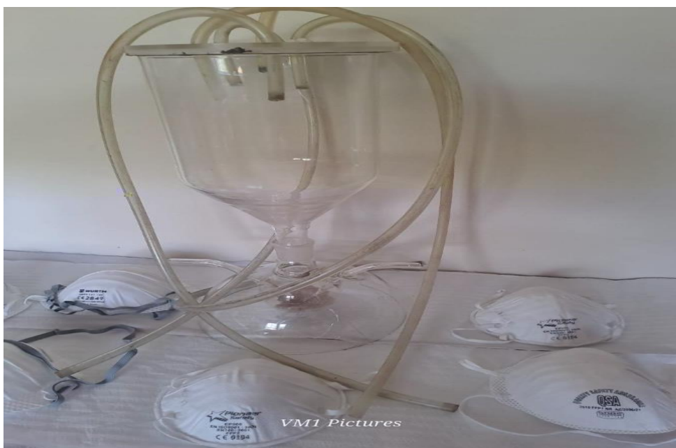
Figure 3.4: Dust masks combined in a dust-generating glass chamber
