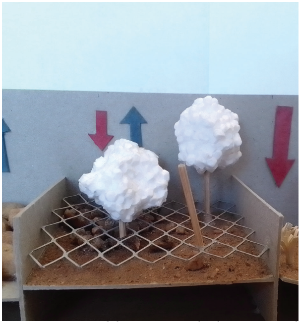
Figure 83: A model comparing the heat gain and evaporation rates of an integrated system used at the FPT University
