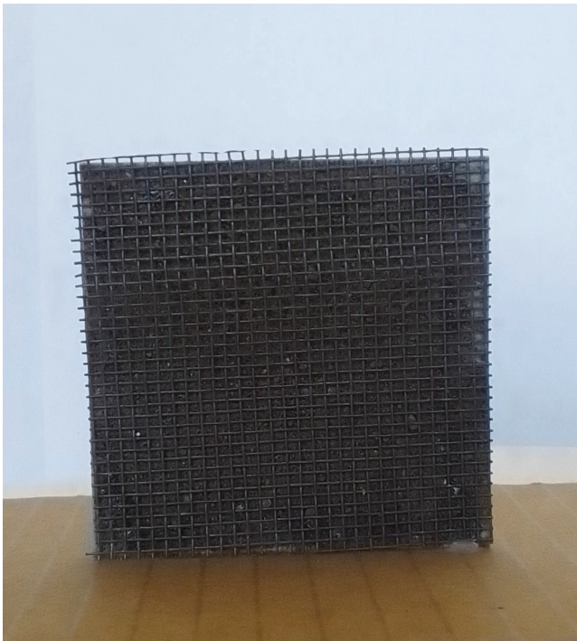
Figure 67: A model of a gabion wall
