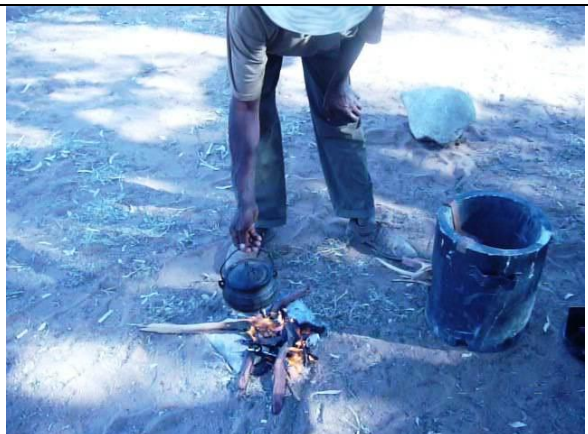
A Tsotso stove saves firewood compared with an open fire.
