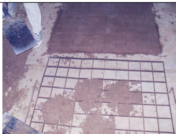
The mixture is then shovelled onto the seed cake mould, to be compacted.
