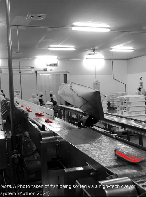
Figure 3.18 High-Tech Fish Sorting
