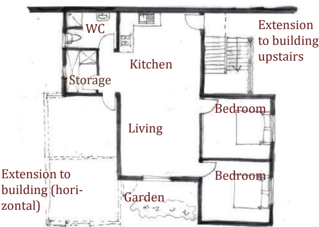
Figure 67: Horizontal upgrade to house Ground Floor (option 1)
