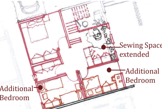
Figure 134: First floor, 22m² built area of stage 2
