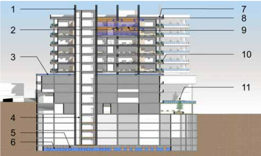
Figure 7.10.5 - South North stacked ventilation section
