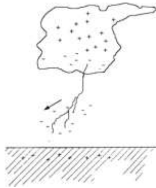
Figure 5: downward negative lightning. adapted from (Akinyemi et al., 2014)
