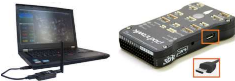
Figure 1 Ground control station and Pixhawk controller, Source 2 :Pixhawk Controller
