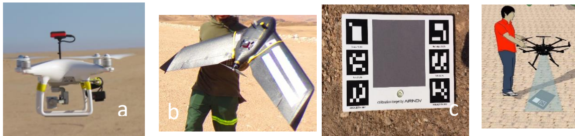
Figure 6. Parrot Sequoia and sunshine sensor mounted on DJI Phantom 4 Professional drone (a) and eBee Classic senseFly drone (b). A standard AIRINOV calibration reflectance target (c), and a Graphic illustrating how to hold the sensor over the calibration target for pre-flight radiometric calibration (d).
