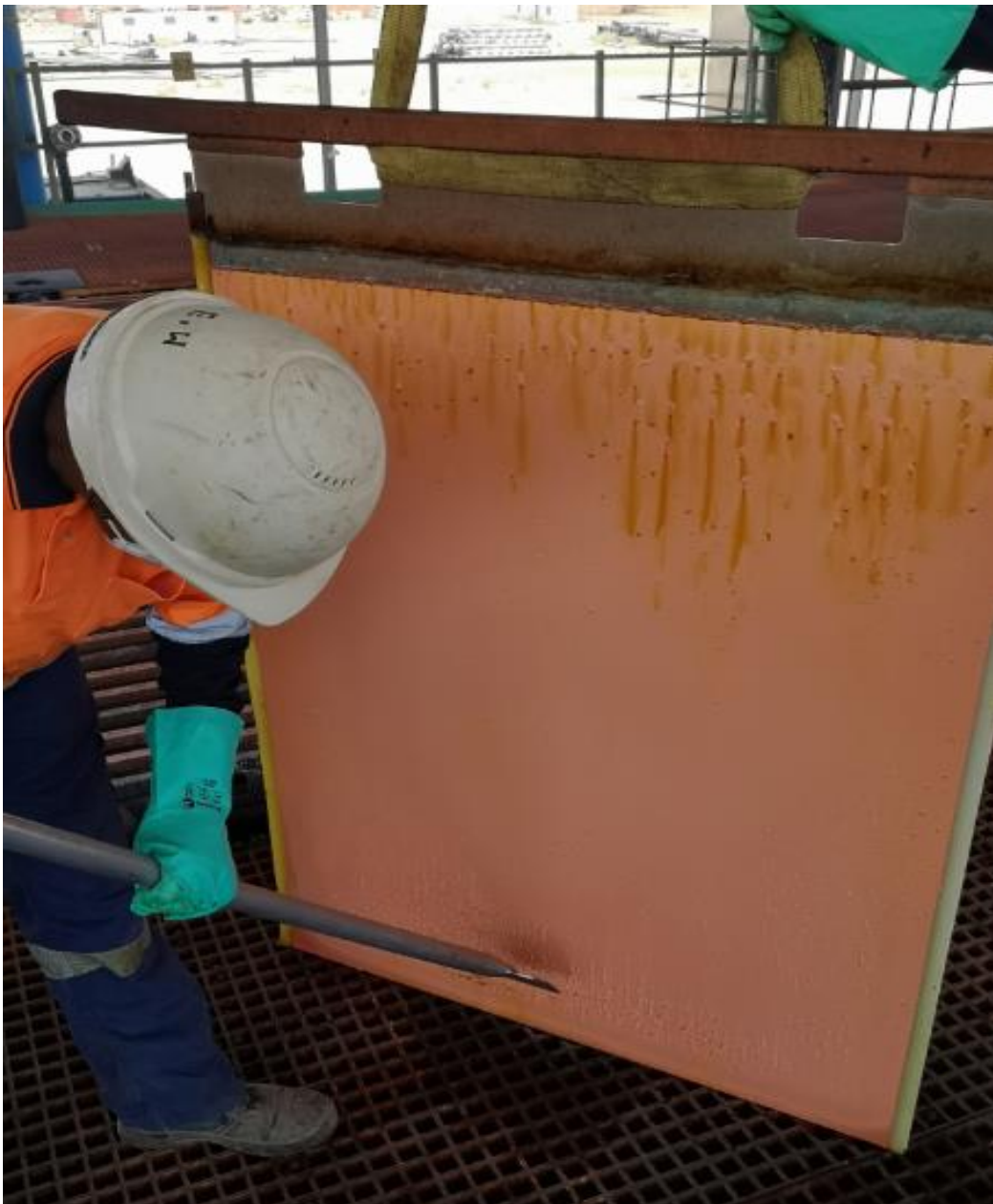
Figure 4.22: Knocking off nodules on a cathode sheet (picture taken by the author)
