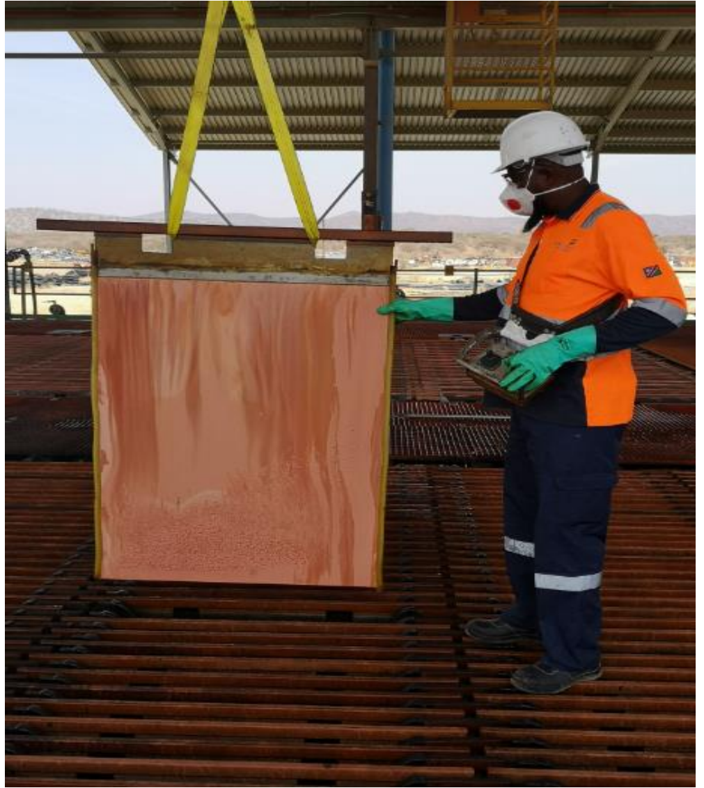
Figure 4.17: Removing a suspected cathode for inspection (picture taken by the author)
