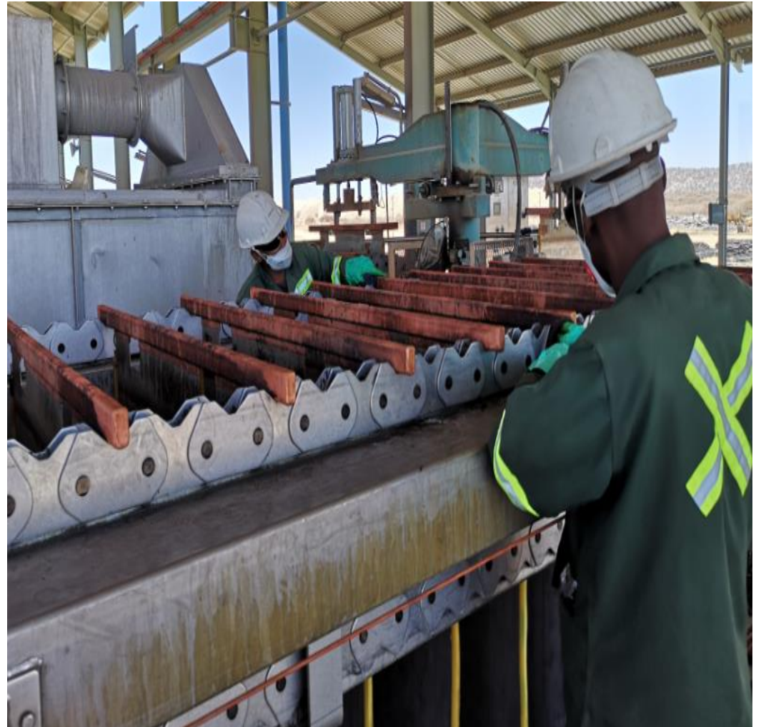
Figure 4.25: Cleaning cathode contacts using acetone (picture taken by the author)
