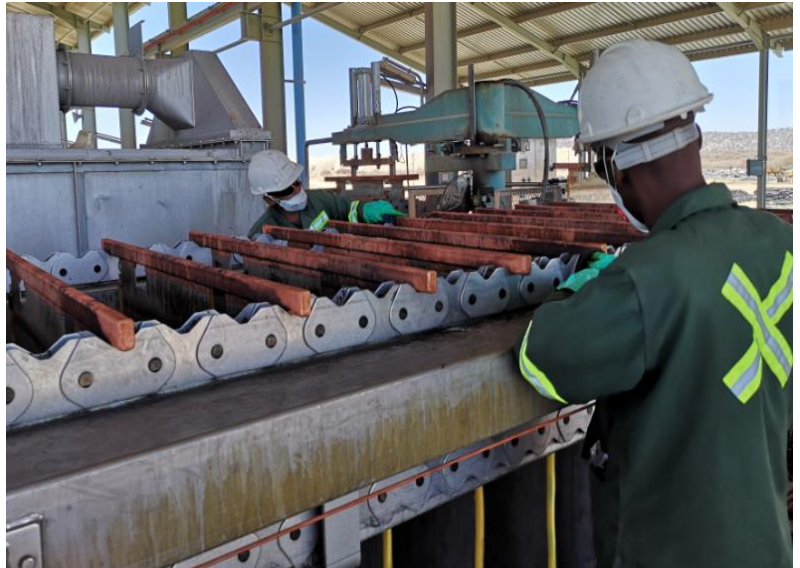
Figure 4.57: Cleaning cathode contacts on the discharge conveyor (picture taken by the author)
