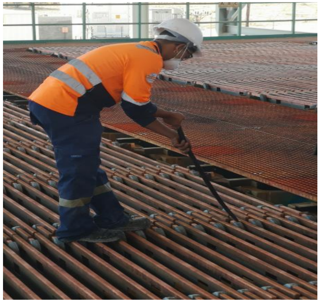
Figure 4.27: Aligning electrodes by doing rat patrol (picture taken by the author)
