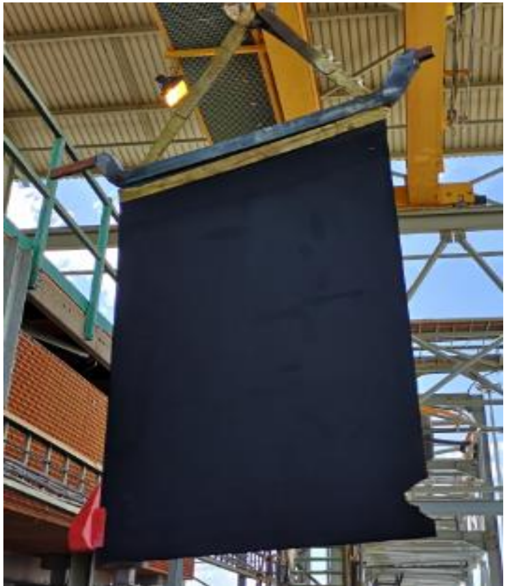
Figure 4.19: A burned anode with a missing side insulator (picture taken by the author)
