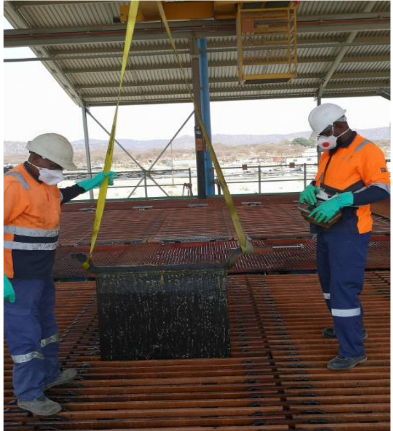
Figure 4.47: Removing an anode from a cell using a sling (picture taken by the author)
