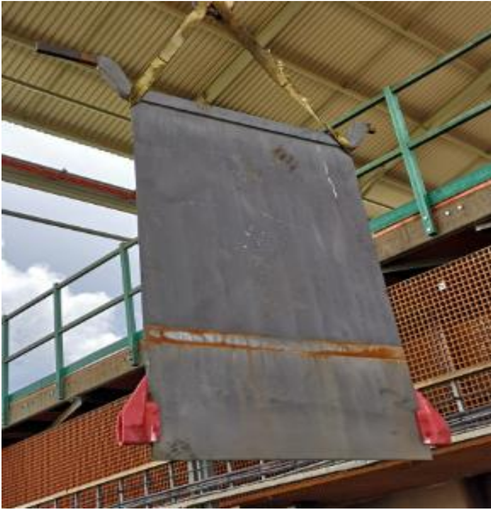
Figure 4.24: Replacing a burnt anode with a brand new anode (picture taken by the author)
