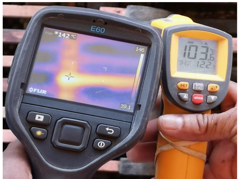
Figure 4.45: Comparing the IR camera to the temperature gun (picture taken by the author)
