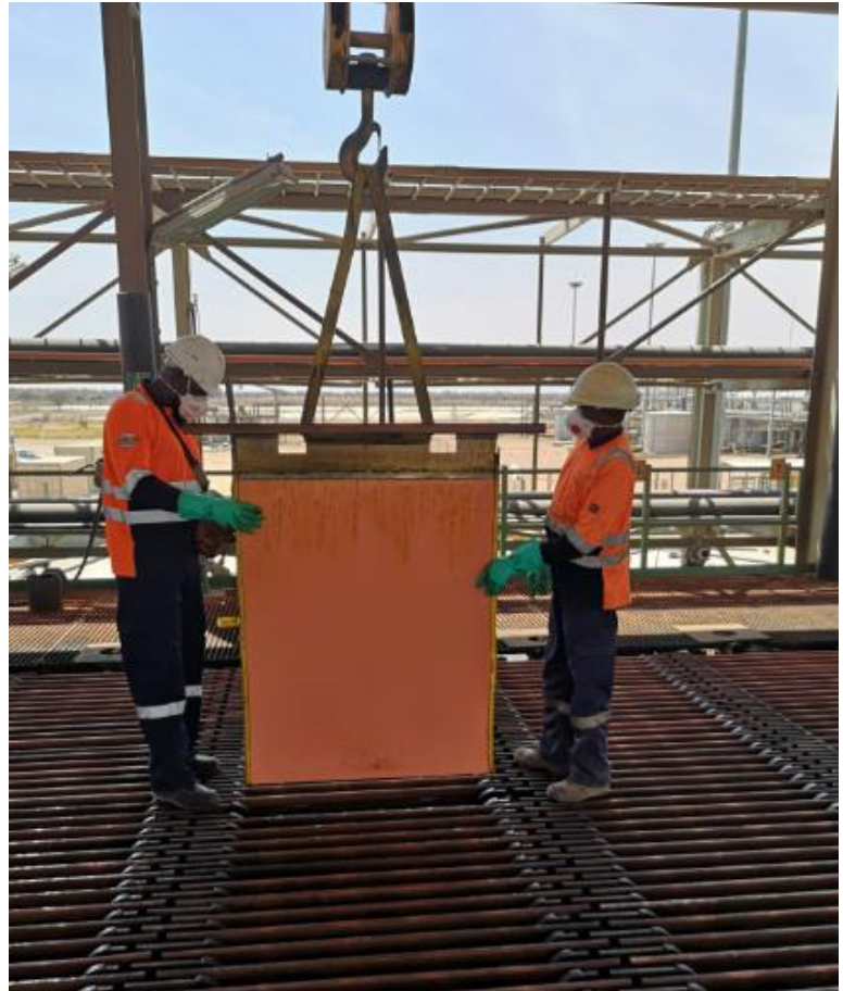
Figure 4.48: Removing a cathode from a cell using a sling (picture taken by the author)
