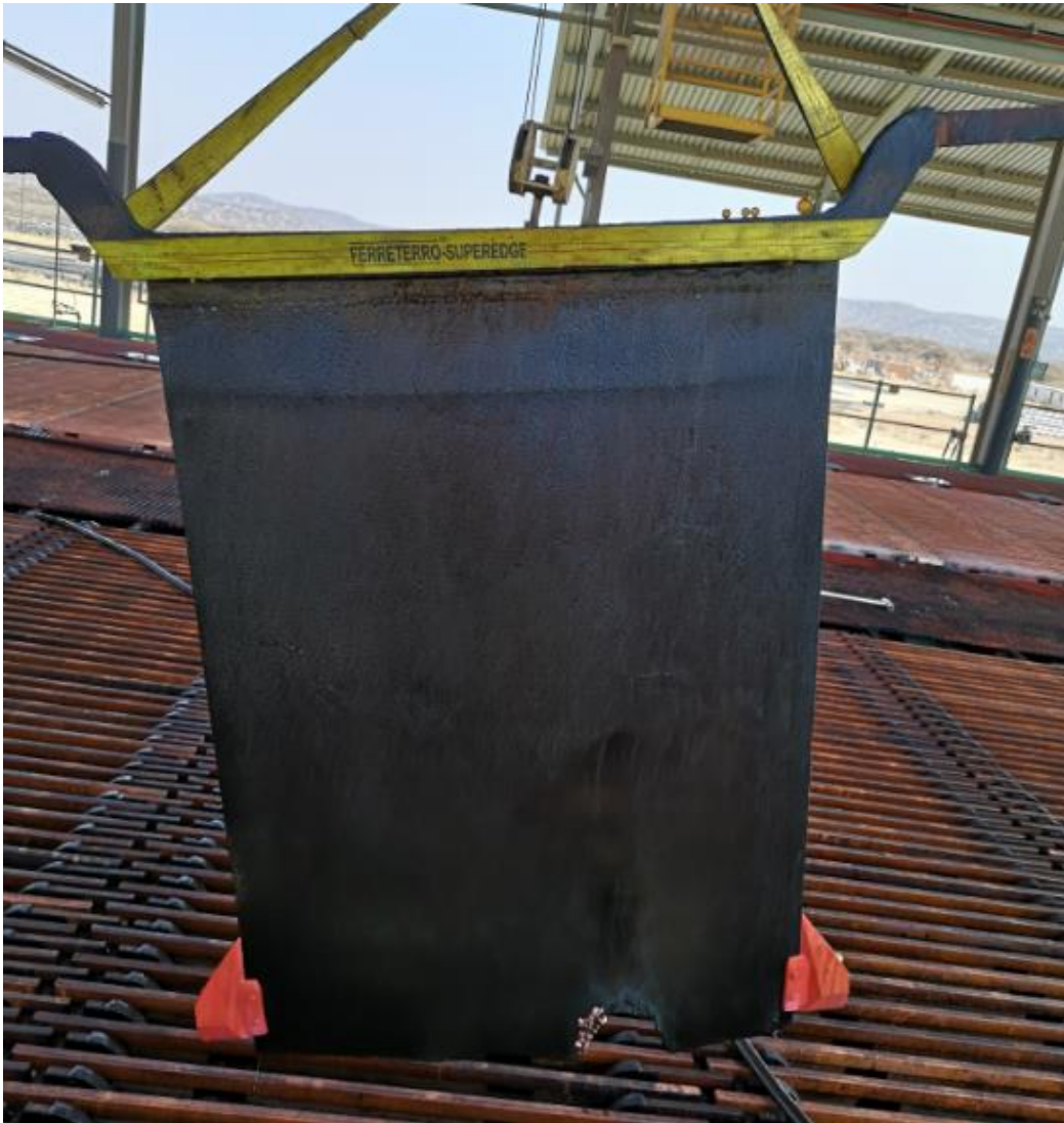
Figure 4.20: A burned anode which was contacting a cathode (picture taken by the author)
