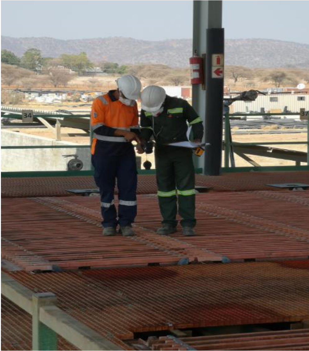
Figure 4.16: Using an IR camera for hotspots detection (picture taken by the author)
