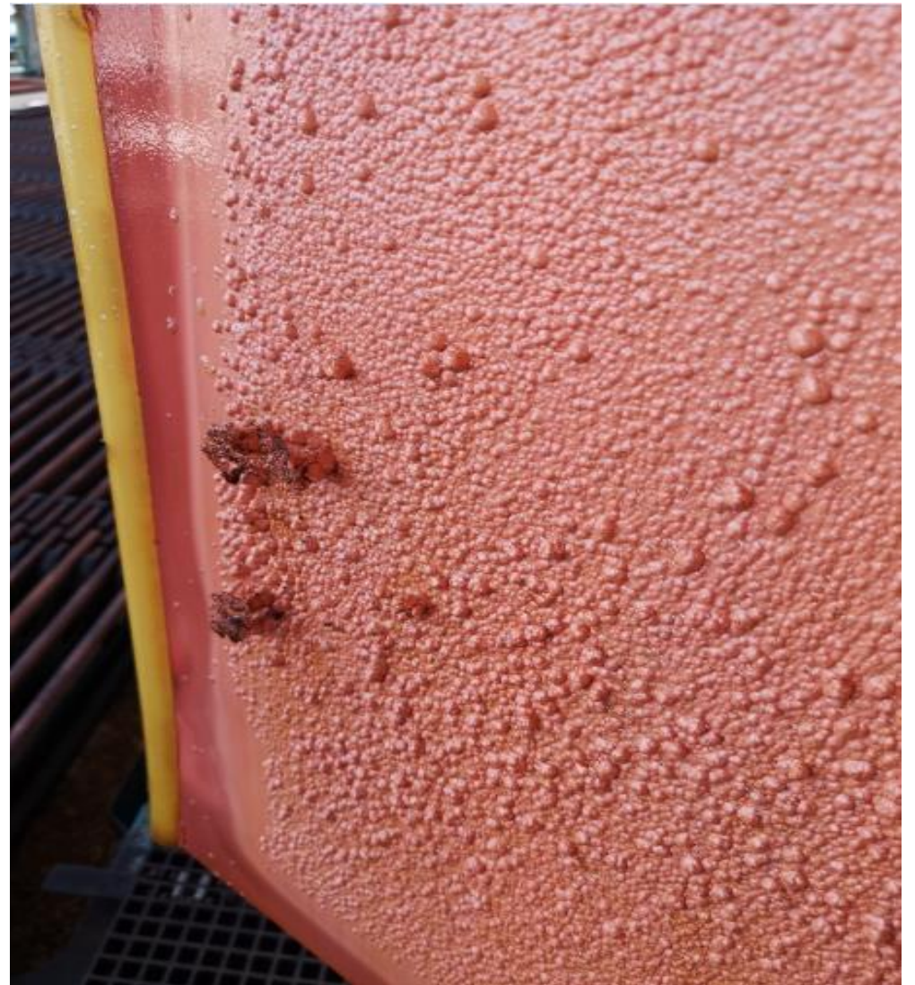
Figure 4.21: Short-circuit due to nodules on a cathode (picture taken by the author)
