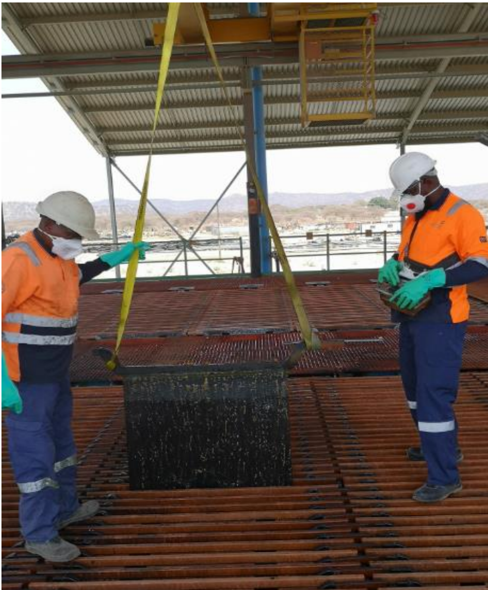
Figure 4.18: Removing a suspected anode for inspection (picture taken by the author)
