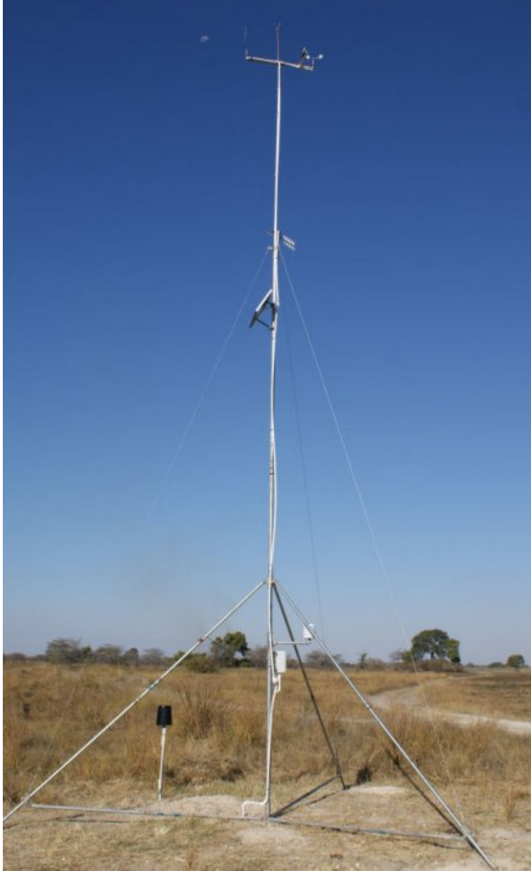
Figure 2: Modified MCS-station as used by the MAWF, on a 10 m pole. This allows the station to fulfil WMO standards. This station is at Kalimbeza in the Zambezi region.
