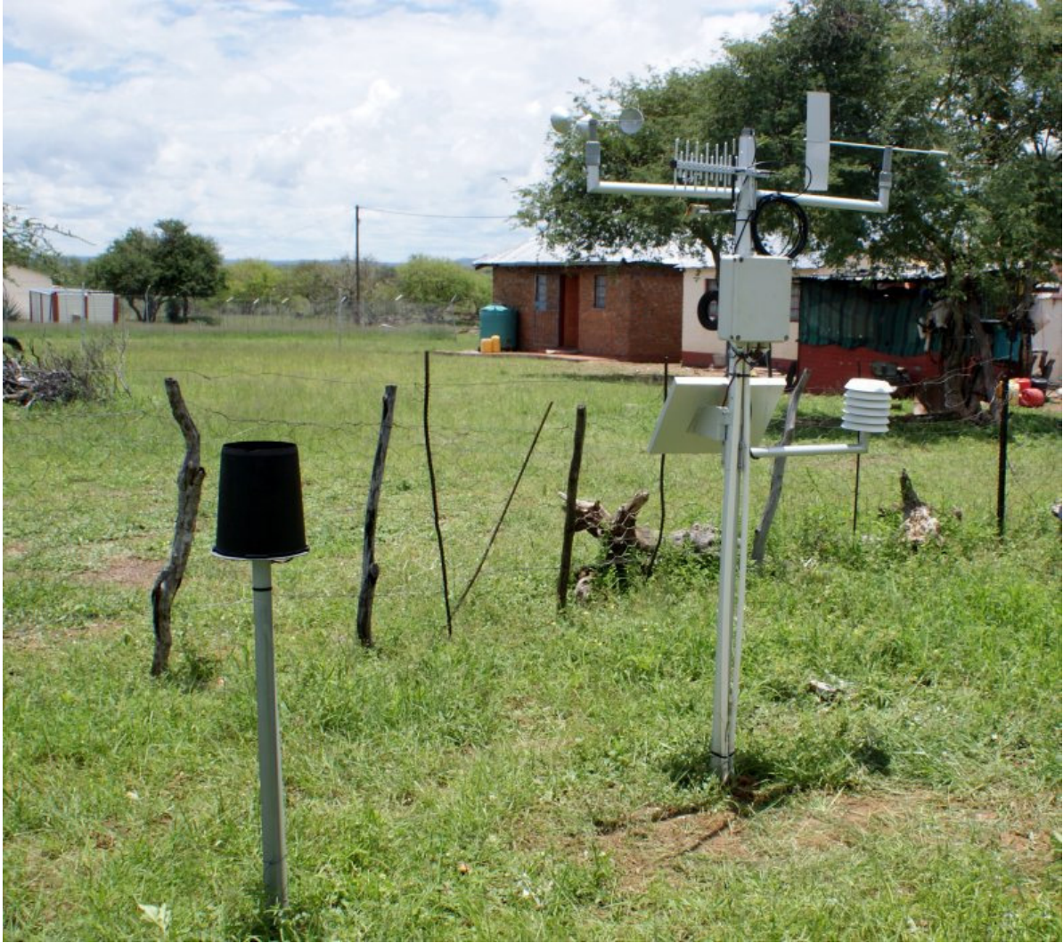
Figure 1: Typical MCS-station, here with Yagi-antenna and solar panel, at Okaboro outside Okahandja.
