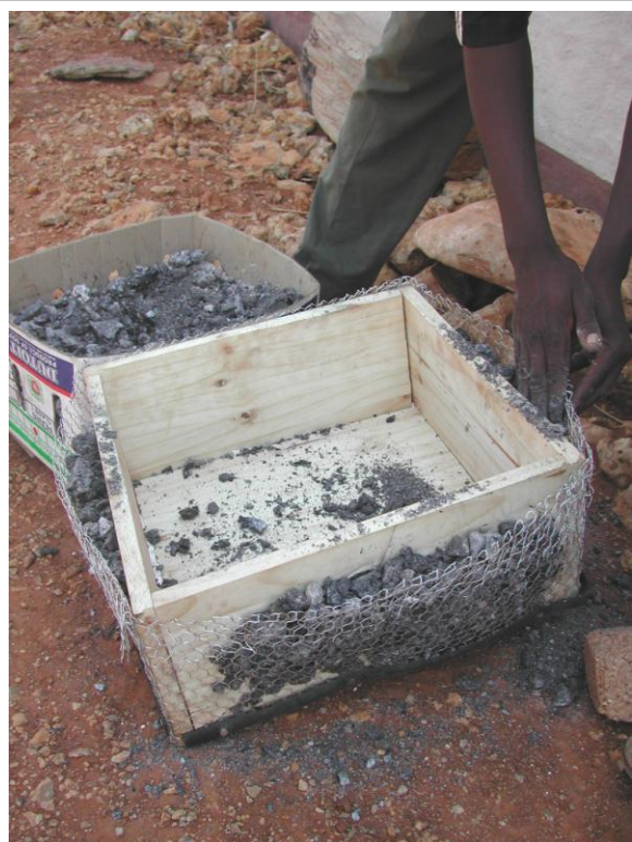
A cool-box is made with charcoal insulation, for evaporative cooling, so that vaccines can be transported for use at the posts.
